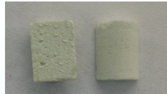
6 mm diameter 10 mm length ~25% porosity
