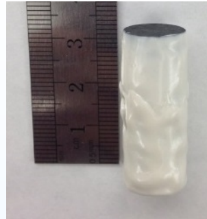
Reassembled Core Wrapped with Epoxy
